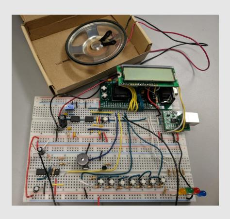
One of the main projects from our undergraduate coursework was to use a microcontroller and other corresponding microelectronics capable of controlling an oven to reflow solder PCB components. I was in charge of writing the assembly code for an 8051 microcontroller we used to control the SSR box connected to the oven.
